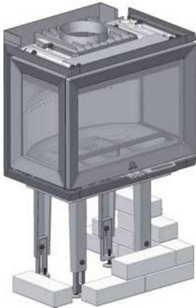
1. The bricks are laid so that they fit under the insert frame.
