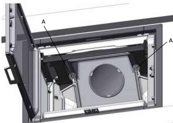
7. Then attach the smoke bell using the screws (A) that had previously been removed when it was taken off the top outlet.
